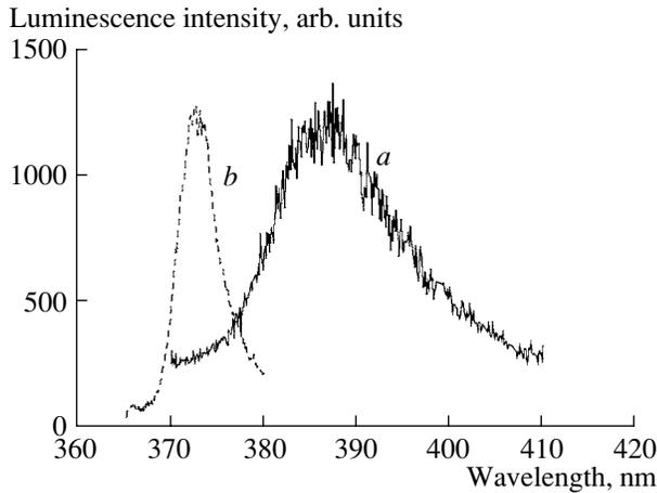
**Fig. 1.** Typical UV-emission spectra of ZnO powders at different temperatures: (a) 300 K; (b) 77 K.
