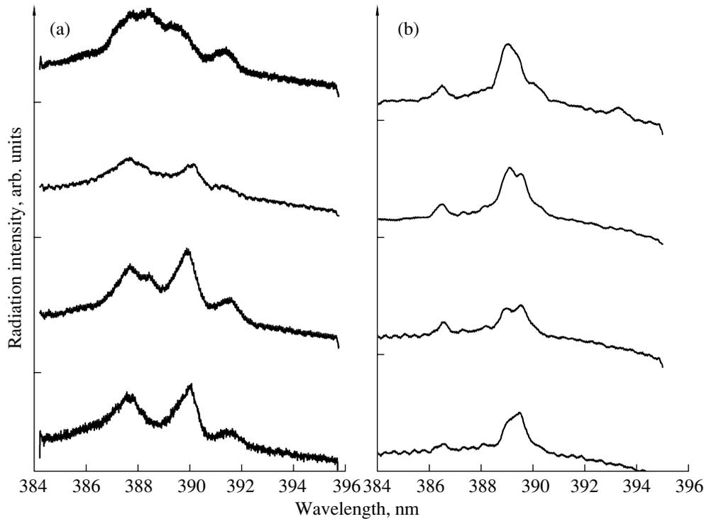
**Fig. 3.** Examples of USA3 lasing spectra: (a) at the first position, (b) at the second position.
