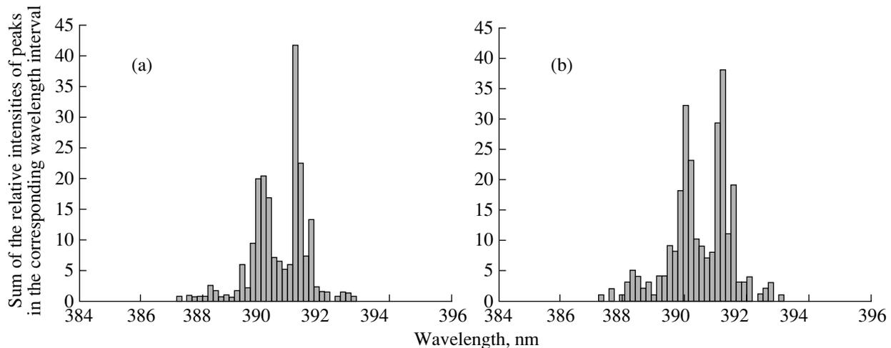
**Fig. 11.** (a) Spectrum of the sum of the relative intensities of peaks of the sample SZ5. (b) Corresponding histogram of the peaks.
