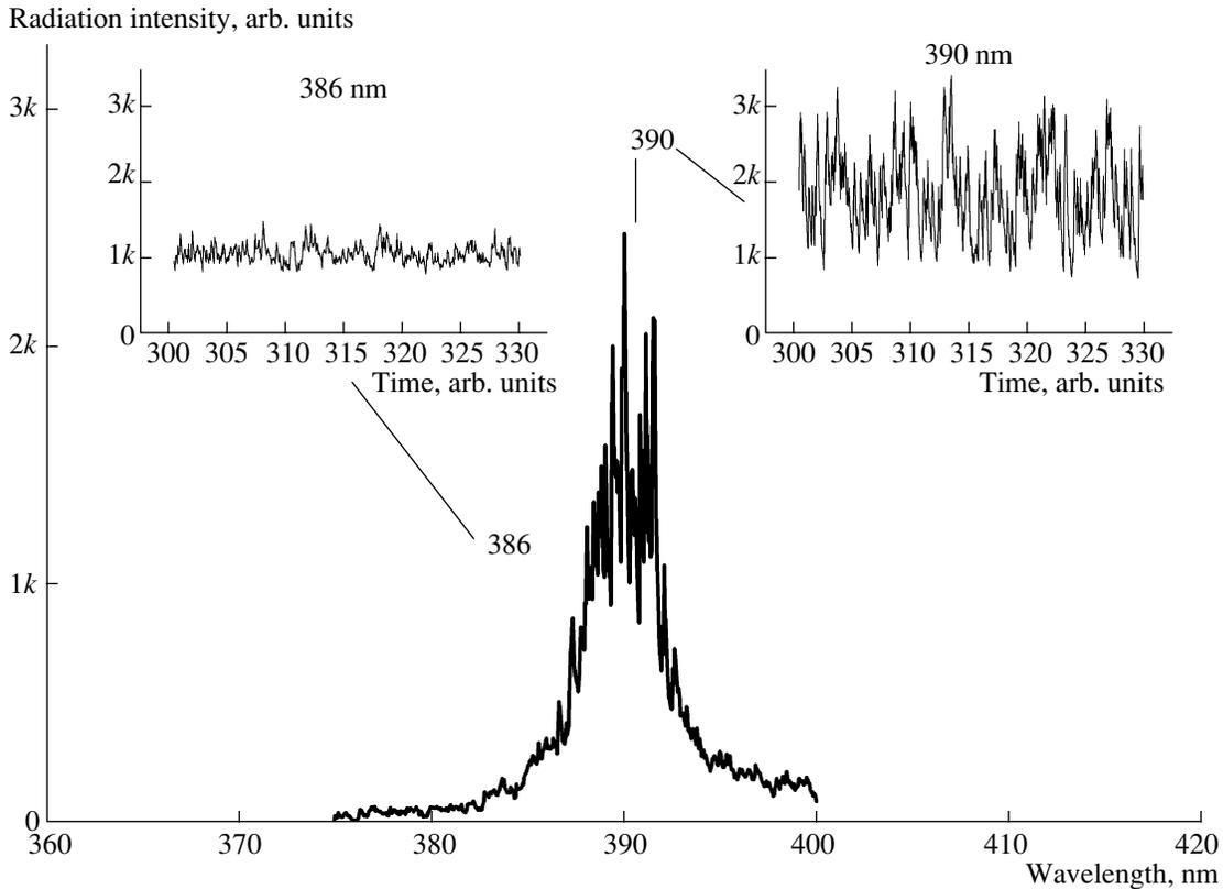
Fig. 1. Lasing spectrum registered with a photomultiplier; insets: time behavior of the signal at a fixed wavelength.
