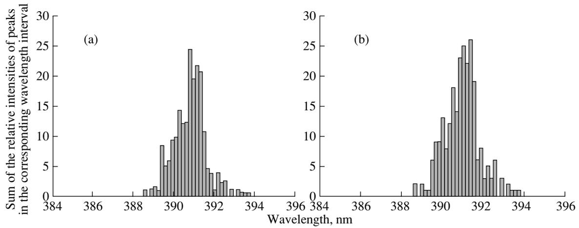
**Fig. 16.** (a) Spectrum of the sum of the relative intensities of peaks of the sample Ch-air700. (b) Corresponding histogram of the peaks.
