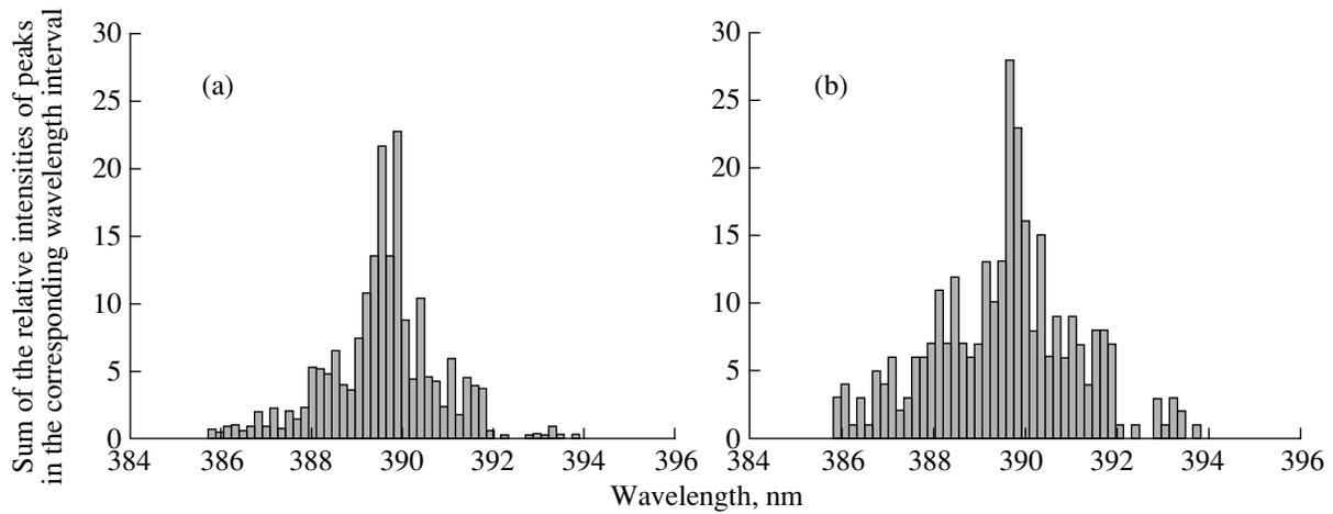
**Fig. 17.** (a) Spectrum of the sum of the relative intensities of peaks of the sample Ch-AR700. (b) Corresponding histogram of the peaks.
